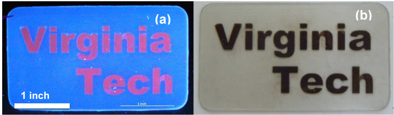
Figure 2-5: QDs Embedding in PolyJet Build under (a) UV light and (b) visible light
